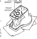
2. Before installing new wax gasket, TEM-PORARILY install flange T-bolts, set toilet, and place discs and nuts onto bolts. Mark bolt length needed for bolt cap clearance
