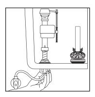
With correct washers in place (see Step 9a), tighten COUPLING NUT 1/4 turn beyond hand tight.
