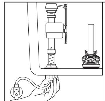
With correct washers in place (see Step 9a), tighten COUPLING NUT 1/4 turn beyond hand tight.
