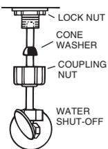
These parts must be used as illustrated to insure water-tight connection. Use of existing coupling nut may result in water leakage. Water supply tube or pipe must extend at least 1/2" inside threaded shank of valve (does not apply to flanged tubing).
