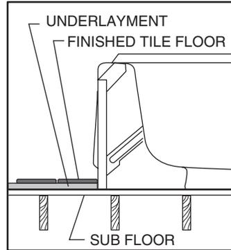
**4** Below is shown typical cross sections of the tub rim showing typical wall constructions.
