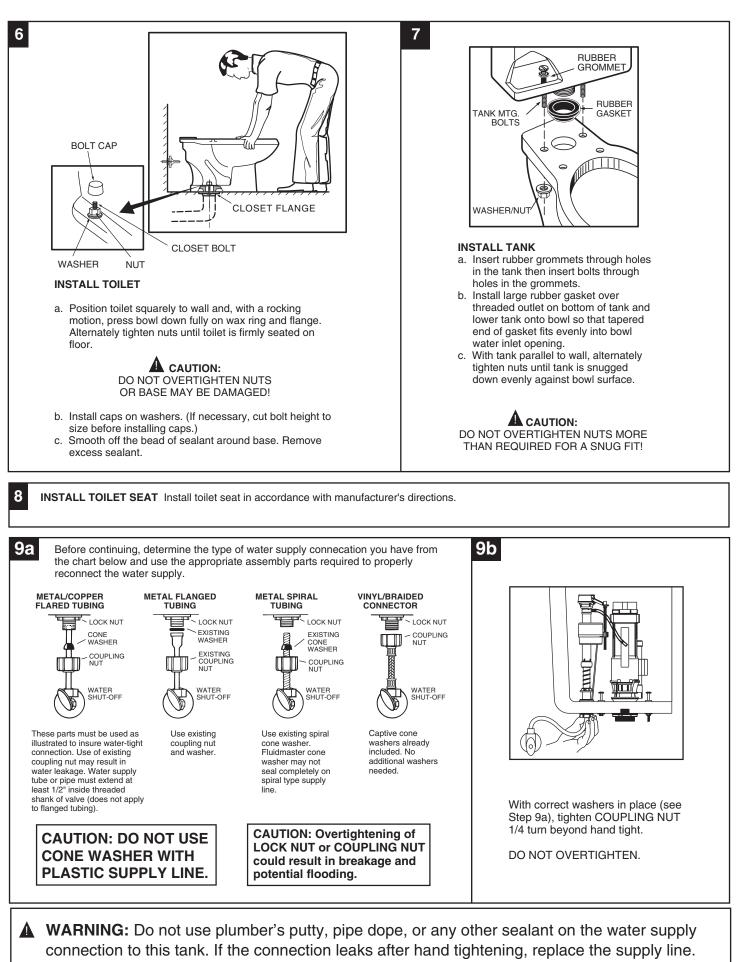
If the connection continues to leak with the new supply line, replace the fill valve.
