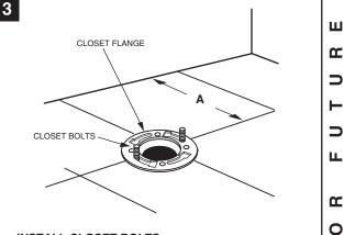
INSTALL CLOSET BOLTS Install closet bolts in flange channel and slide into place parallel to wall.
