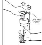
IMPORTANT: Always clear sand and rust from system. Make sure water supply is off. Remove valve TOP by lifting arm and rotating top and arm 1/8 turn counterclockwise, pressing down slightly on cap.
