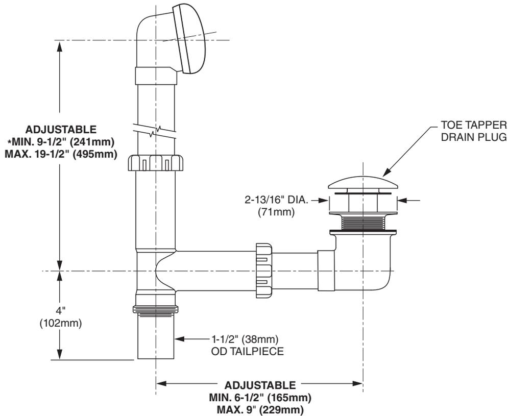
\* NOTE: For overflow heights less than 17" (432mm), cutting the pipe is required.
