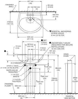
NOTES: \* DIMENSIONS SHOWN FOR LOCATION OF SUPPLIES AND "P" TRAP ARE SUGGESTED. ▼ANCHOR SCREWS FOR PEDESTAL NOT INCLUDED. INSTALLATION INSTRUCTIONS SUPPLIED WITH LAVATORY.
